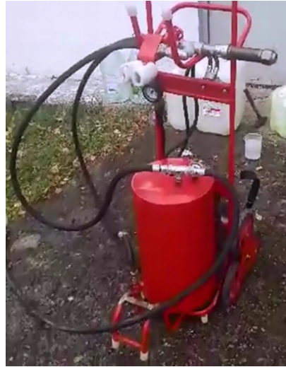
Fig. 1. Experimental mobile installation for the generation of compression foam
