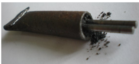
Fig. 4. Samples – korneisen placed in container with carbonizer composition of 50 % graphite and 50 % soda ash
