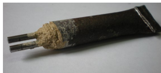
Fig. 5. The samples in container with airtight clay gate
