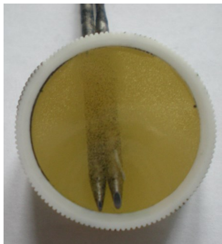
Fig. 7. Microsection prepared for metallographic analysis
