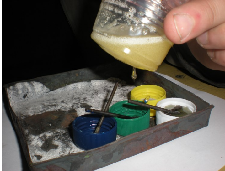
Fig. 6. Filling the samples with epoxy glue
