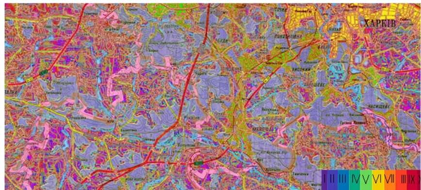
Fig. 5. Graphical interpretation of the calibration of the local area according to the calculated level of fire danger
