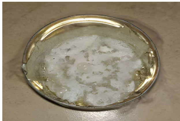
Figure 3. Contaminated JET A-1 aviation fuel (source: Authors, 2022)
