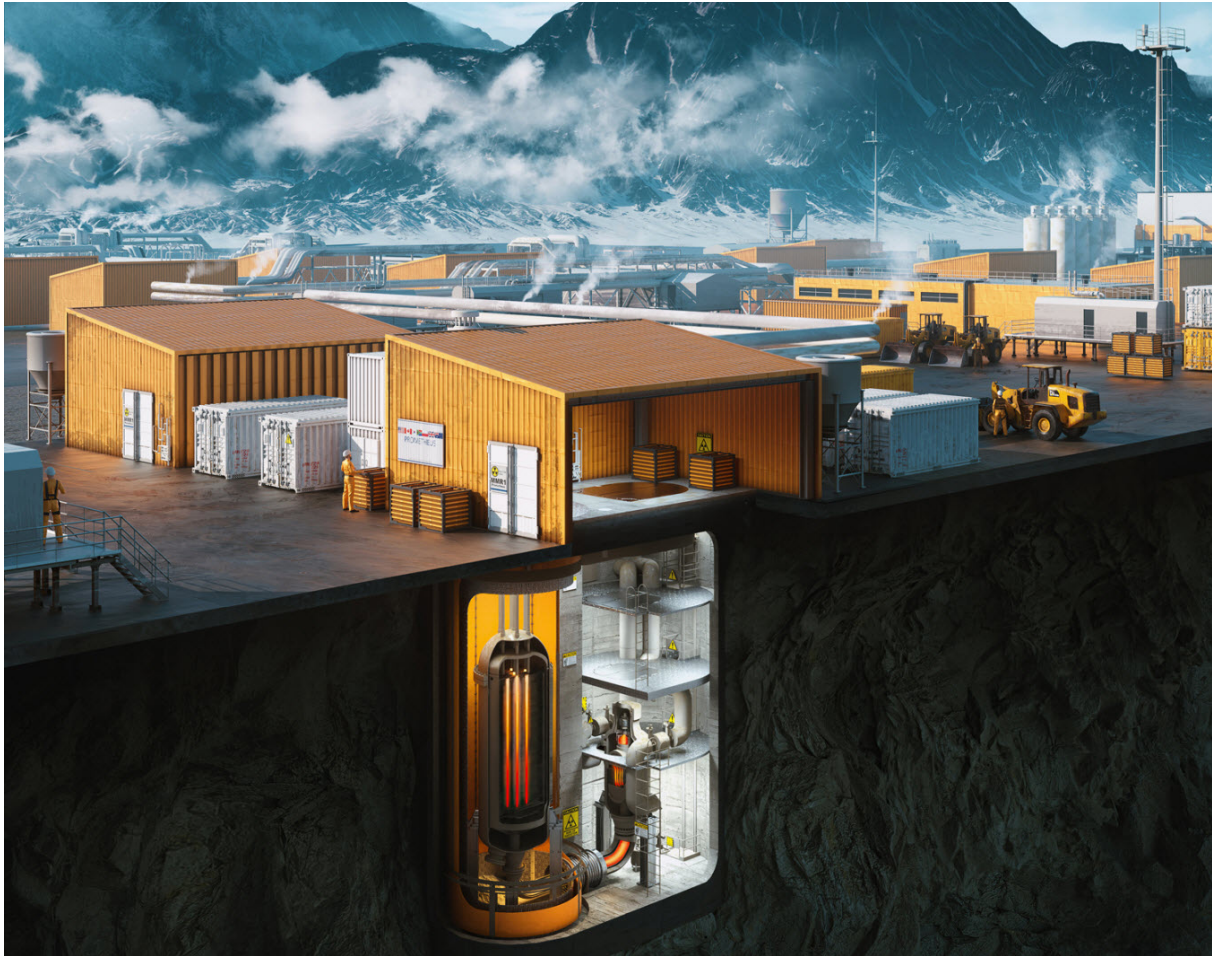
Figure 3. Example of underground placement of SMR [53].
