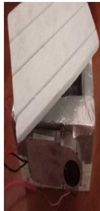
Fig. 5. Appearance of the test prototype of the refrigerating chamber
