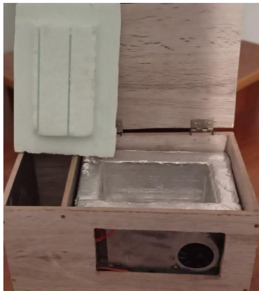
Fig. 6. Appearance of the test prototype of the mini-refrigerator
