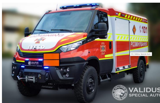
Fig. 1 – PM-L based on the IVECO DAILY 55S
