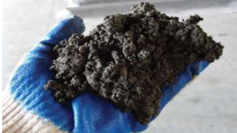
Fig. 2. Roller Compacted Concrete mixture. Source: private collection.
