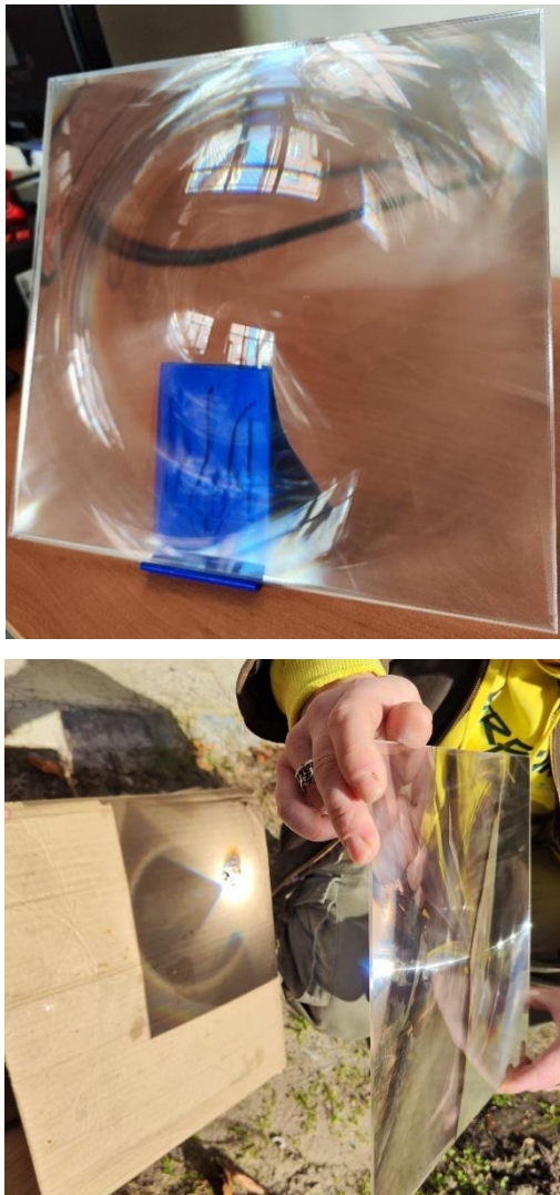
Fig. 5 – Concentrating system based on a Fresnel lens
