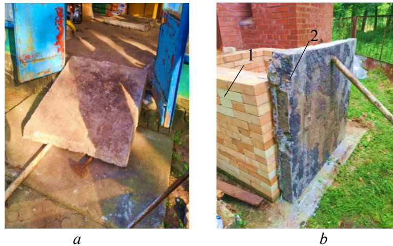
Fig. 1. A small fragment of a reinforced concrete wall made in advance of the test: a – transportation of the fragment; b – a fragment of the wall installed at the test site, before the test; 1 – walls of the fire furnace; 2 – fragment of reinforced concrete wall for testing
