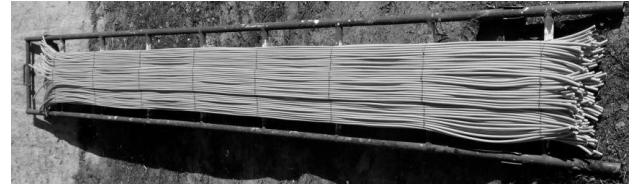
Fig. 4. Cable physical appearance in a special frame to form a bundle of A category based on [1]
