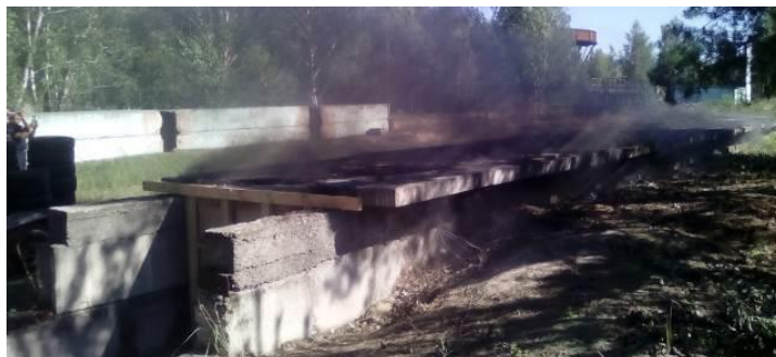
Fig. 10. Photograph of the cable tunnel in the course of the experiment
