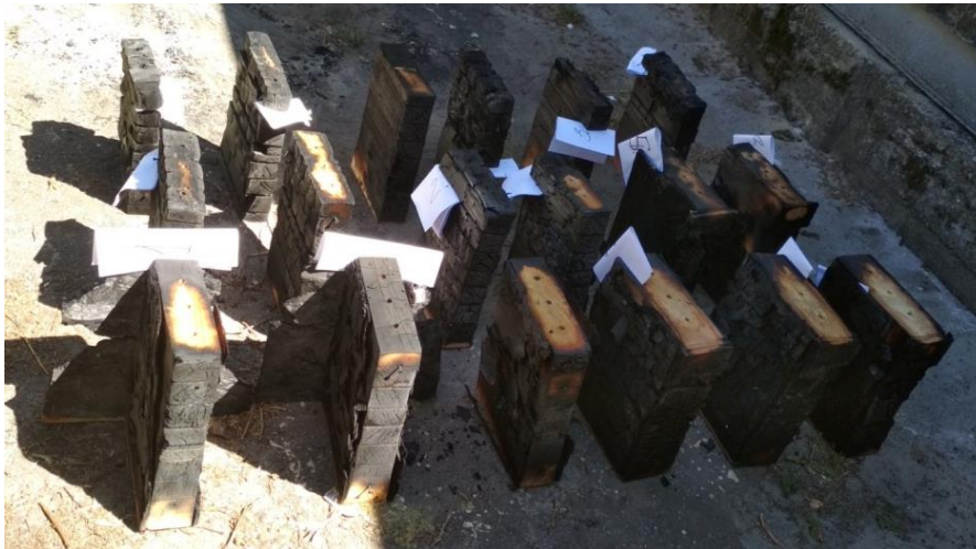
Figure 1 – Photo samples after fire tests
