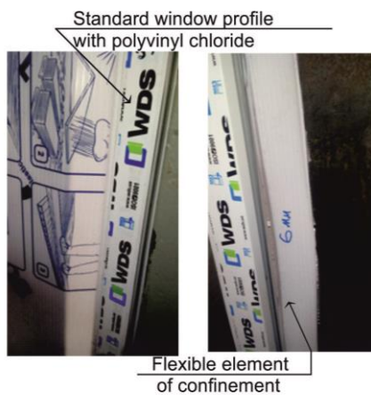
Fig. 1: The view of the glazing element of the researched relief panels (RP) system.
