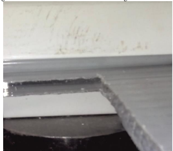
Fig. 3: The view and internal structure of a sheet of the fencing flexible element.
