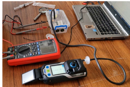
Fig. 2. Laboratory setup for studying the effect of relative humidity of the atmospheric air on the working parameters of the gas sensor
