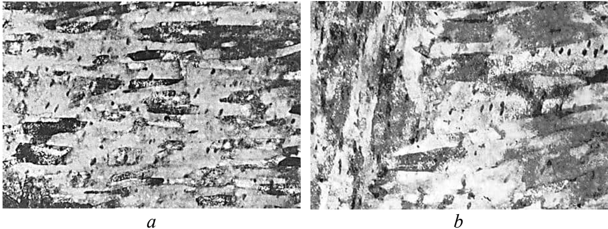
Figure 5 - Structure of St3kp steel, transformation temperature 400\ ^\circ\text{C} a, b – electron microscopic magnification \times 14000
