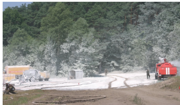
Fig. 4. Extinguishing of gas blowout fire by using a powder jet Source: Own elaboration.
