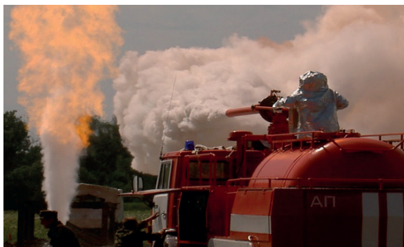
Fig. 4. Extinguishing of gas blowout fire by using a powder jet Source: Own elaboration.
