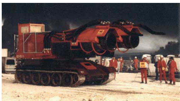
Fig. 3. Gas/water jet extinguishing vehicles [17], [18], [21]
