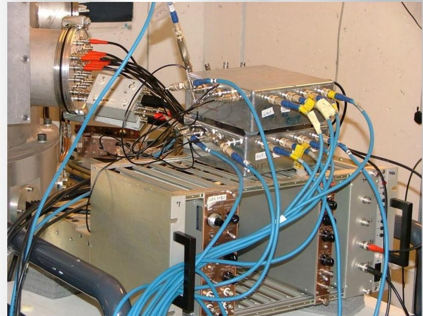
Figure 3. Front-end electronics in the experiment cave outside the vacuum chamber.
