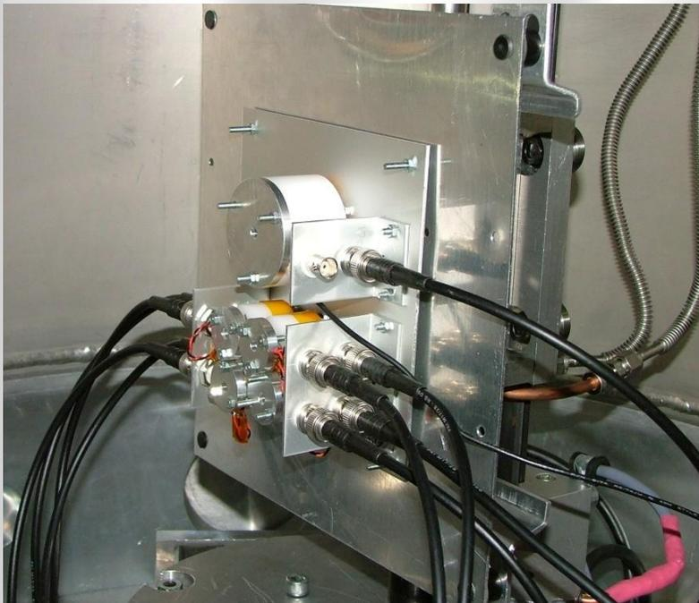
Figure 2. Performance test detectors in the vacuum chamber.
