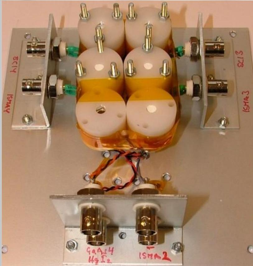
Figure 6. Detector test fixture used in the radiation tests.
